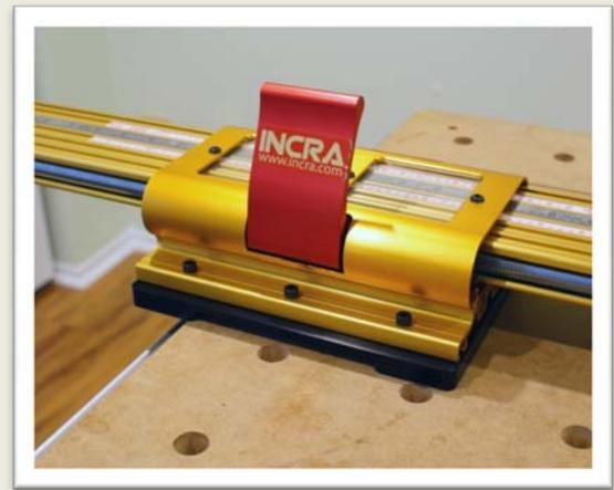
3. Next step is securing Incra-LS Positioner with a Precision Plate to your MFT/3 (or other custom workbench with a condition that holes 96mm from each other) with our knobs or Festool knobs with M8 bolt.
