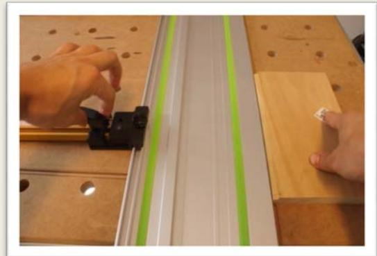
6. Slide tape measure on a T-Track until 0 (zero) is aligned with a side of a Length Adapter opposite to the guide rail. Once this is done, your system has been calibrated and scales adjusted.
