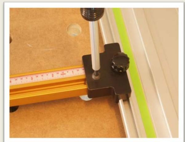
4. To calibrate Precision parallel guides, slide the Length Adapter until it hits the Guide rail bracket (spacers should appear under your guide rail as seen on the second picture below).
