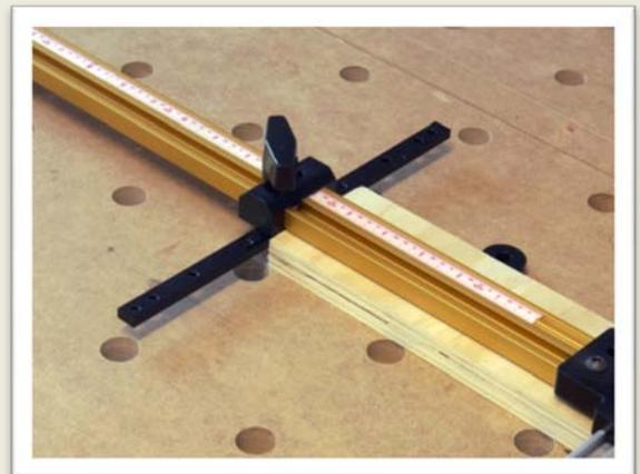
install one Spacer on two Length Adapters (this ensures that T-Tracks stay parallel no matter how far from guide rail they are, thus contributing to accuracy for ripping widest pieces).
