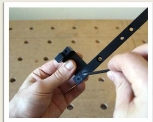
2. Install a Guide Rail bracket by sliding it from the side of the guide rail.
