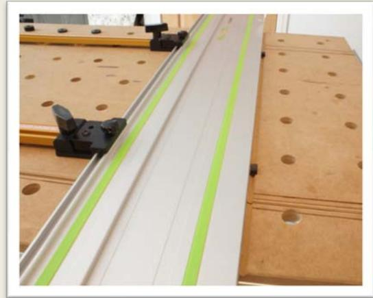
5. Using a short straight edge or a block of wood with a side perpendicular to its surface press against the spacer until your straight edge hits the guide rail's splinter guard strip. Once it does, tighten a thumbscrew on the Length Adapter and repeat the same steps with the second spacer.
